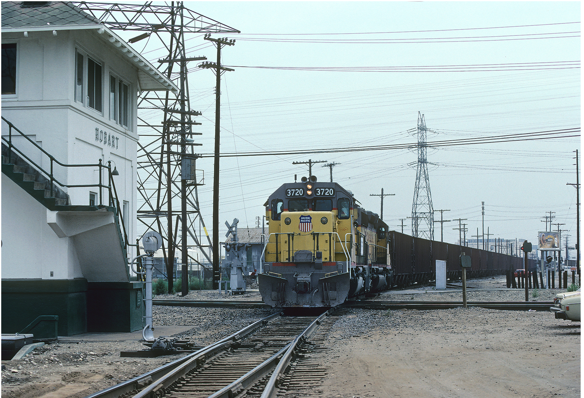
A UP empty coal unit train crosses Santa Fe's main line at Hobart Tower in Vernon, 10 August 1983. At the time, the Santa Fe main line at Hobart hosted 35 through train movements per day plus frequent switching moves. With the planned introduction of commuter service, the train count on the Santa Fe tracks would more than double. UP trains stopped for conflicting Santa Fe movements blocked multiple city street crossings.
