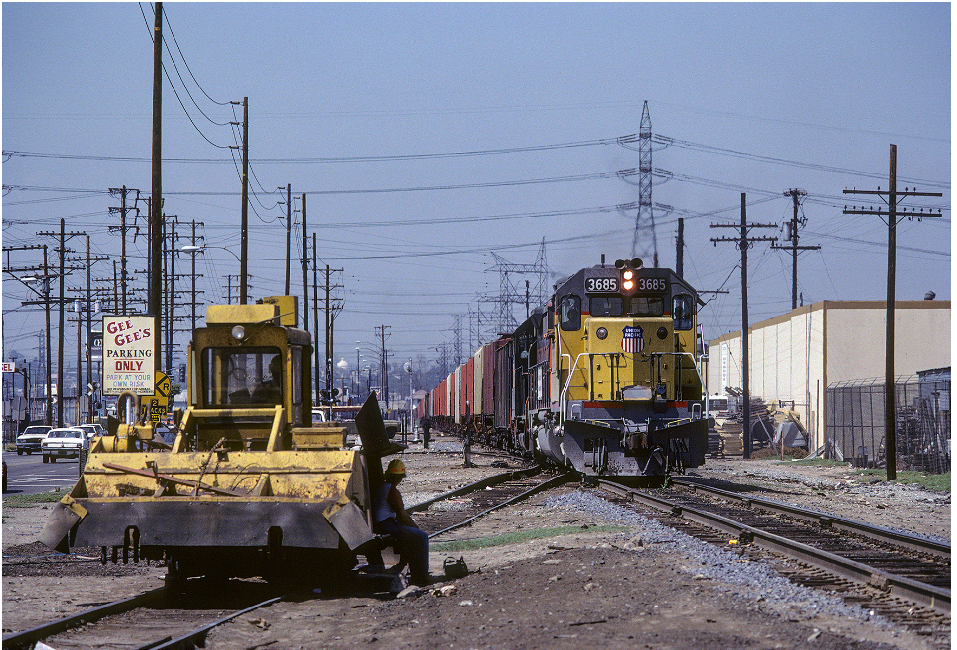
A UP potash unit train passes through the automatic interlocking governing the crossing of the Los Angeles Junction Railway in Vernon, 10 August 1983. Maintenance of way equipment stands in the clear on an industrial support drill track.
