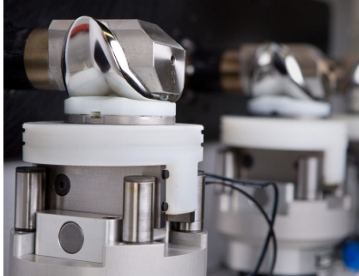
Figure 19: The commercially available ADL knee simulator controls dynamic loading, flexion, internal-external rotation, and anterior-posterior translation, with free motion allowed in medial-lateral translation and valgus rotation (AMTI n.d.).
