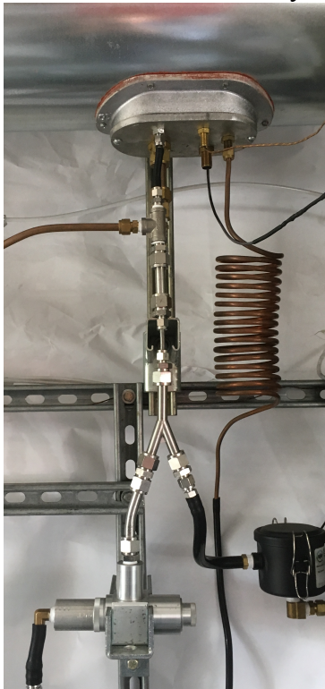
Figure A14. Photograph of secondary diluter at Lawrence Berkeley National Laboratory (left) and cut-section of the diluter as built (right). The diluter is entirely constructed from plumbing parts, and volumetric flow rates are controlled using Alicat Scientific mass flow controllers
