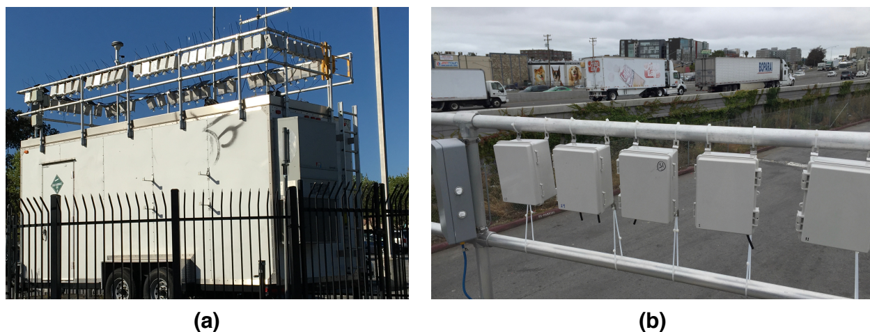
Figure C1. (a) Over 60 Aerosol Black Carbon Detector (ABCD) units hung from the railing of the Bay Area Air Quality Management District (BAAQMD) roadside monitoring station in Oakland, California; (b) Close up view of ABCD units deployed at the monitoring station, with California Highway 880 in background.
