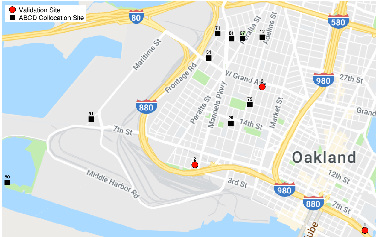
Figure D4. ABCD collocation sites in the 100×100 Network. At validation sites, four ABCD units were deployed in collocation with a commercial BC monitor (Model AE33, Magee Scientific). At collocation sites, ABCD units were deployed in pairs. Major roads and highways are also labeled for reference.
