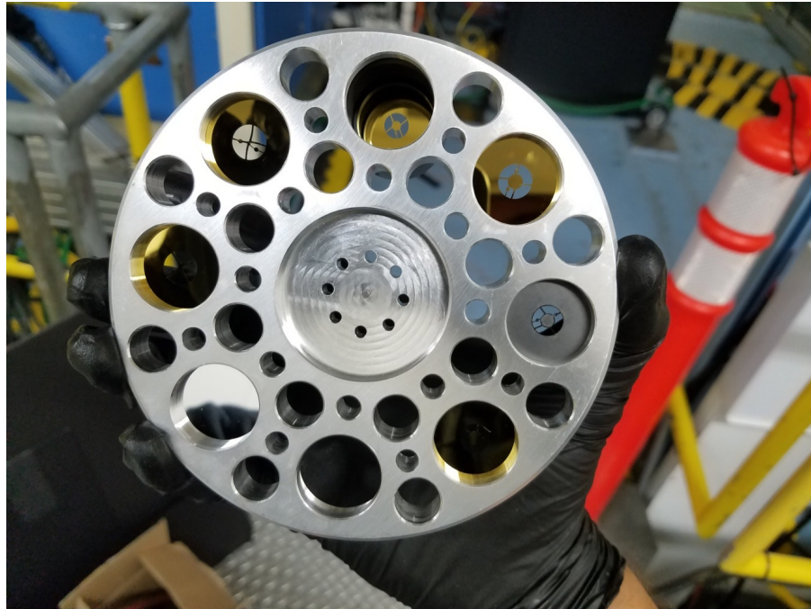
Figure 1.4 Picture of Lyot stops in the SCEXAO filter wheel that we fabricated in 2018. Picture credit: J. Lozi
