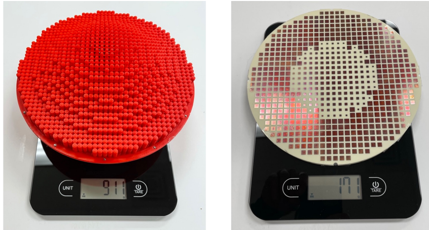
Figure 4.14 Weight Comparison of 18 cm 3D-printed lens that was presented in chapter 2 and the 18-cm transmitarray (both operate at 13.4 GHz). The measured weight of the transmitarray is 0.171 kg, which is less than 20% of the weight (0.911 kg) of the 3D-printed lens of the same diameter.
