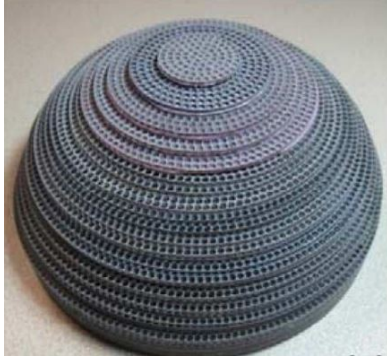
(a) Half-spherical Luneburg lens antenna based on the drilled-hole approach on the commercially available dielectric boards [12].
