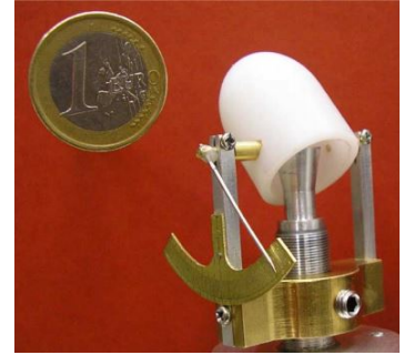
(c) Compact Beam-Steerable Lens Antenna for 60-GHz WirelessHD Communications [6].
