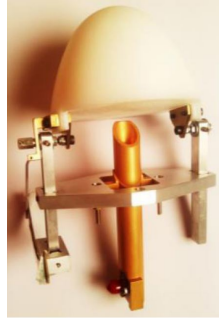
(b) Stereolithography-Based Antennas for Satellite Communications in Ka-Band [5].
