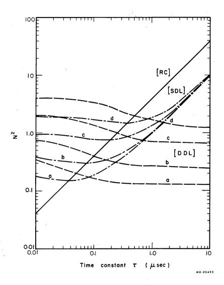
Fig. 11. Normalized effective-energy-squared equations from current noise, expressed as  $E_{eff}^2 = 3.9 \times 10^{13} \text{ N}^2 \text{I} (\text{ev}^2)$ , where I is in amp. The shaping curves were developed from the following formulas:
