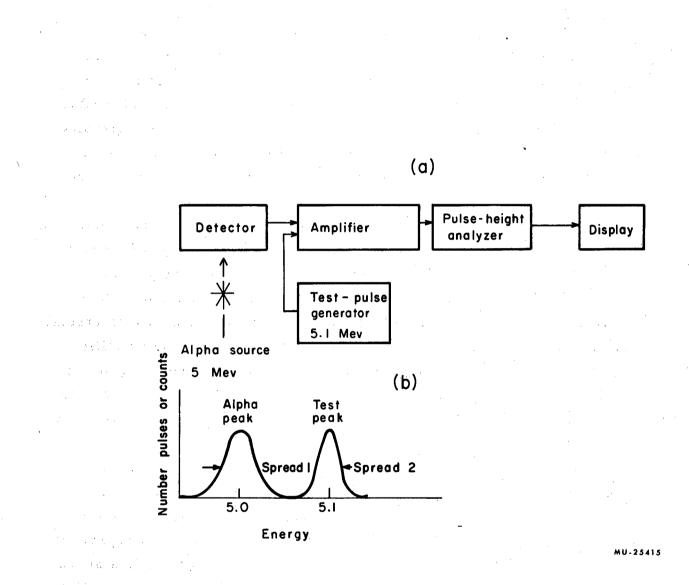
Fig. 1. (a) Block diagram of a system for measuring alpha particles. (b) Distribution of pulse amplitudes from the pulse-height analyzer.
