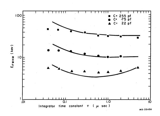
Fig. 19. Calculated and measured resolution curves for single-delay-line shaping. Parameters are
