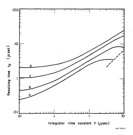
Fig. 14B. Resolving time for double-delay-time shaping for delay-line times  $(2\tau_0)$  of 0.1 (a), 0.2 (b), 0.5 (c), and 1.0 (d) µsec, with an amplitude error (P) of 1.0%. The restriction that  $t_p > 4 \tau_0$  does not hold for integrator time constants to the right of the dashed line.
