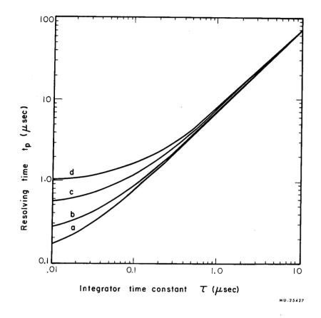
Fig. 13A. Resolving time for single-delay-line shaping. Curves have been plotted for delay times  $(2\tau_0)$  of 0.1 (a), 0.2 (b), 0.5 (c), and 1.0 (d) µsec, as indicated, with an amplitude error (P) of 0.1%.
