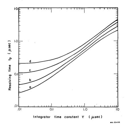
Fig. 14A. Resolving time for double-delay-time shaping for delay-line times  $(2\tau_0)$  of 0.1 (a), 0.2 (b), 0.5 (c), and 1.0 (d)  $\mu$ sec, with an amplitude error (P) of 0.1%.
