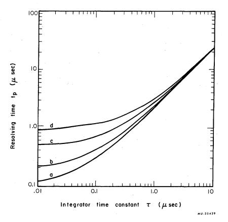
Fig. 13C. Resolving time for single-delay-line shaping. Curves have been plotted for delay times  $(2\tau_0)$  of 0.1 (a), 0.2 (b), 0.5 (c), and 1.0 (d) µsec, as indicated, with an amplitude error (P) of 10%.
