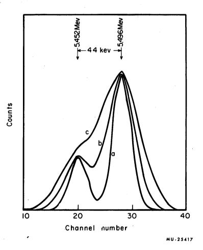
Fig. 3. Energy spectrum of Pu<sup>238</sup> (two alpha peaks) for FWHM energy resolutions of (a) 20 kev, (b) 30 kev, and (c) 40 kev. The energy of each channel is approx 11 kev.
