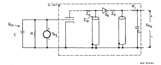
Fig. 27. The equivalent noise circuit of the amplifier for double-delay-line shaping. C denotes the detector and tube-input capacitances, and R is the resistance from grid to ground.
