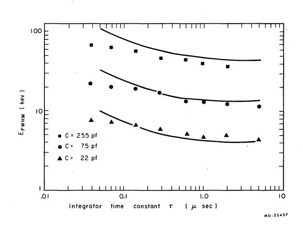
Fig. 20. Calculated and measured resolution curves for double-delay-line shaping. Parameters are
