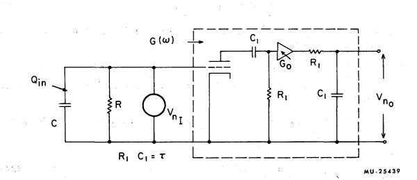
Fig. 22. Equivalent noise circuit of the amplifier for RC shaping. C denotes the detector and tube-input capacitances, and R is the resistance from grid to ground.
