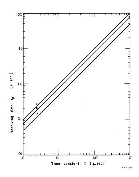
Fig. 12. Resolving time for RC shaping, plotted with amplitude errors (P) of 0.1% (a), 1.0% (b), and 10% (c). The curves were developed from
