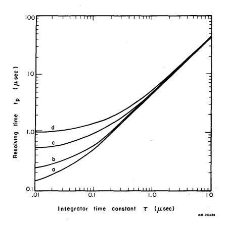
Fig. 13B. Resolving time for single-delay-line shaping. Curves have been plotted for delay times  $(2\tau_0)$  of 0.1 (a), 0.2 (b), 0.5 (c), and 1.0 (d) µsec, as indicated, with an amplitude error (P) of 1.0%.
