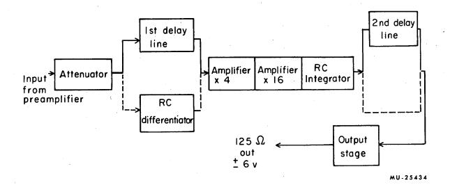
Fig. 17. Block diagram of the post amplifier.
