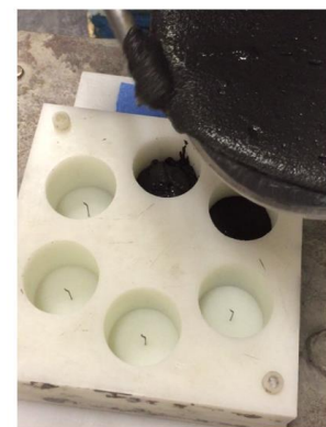
Figure 58: Casting of single fiber pull-out specimen
