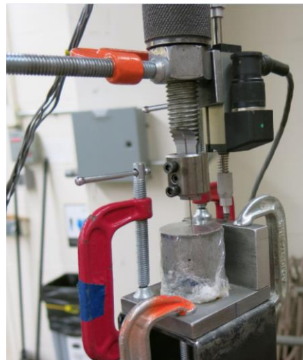
Figure 60: Close view of single fiber pull-out test set-up for the specimen glued to a steel plate.
