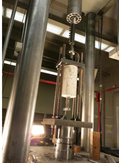
Figure 23: Set-up for conventional rebar pull-out test with cyclic loading protocol
