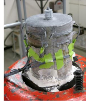
Figure 44: Support condition of modified pull-out test
