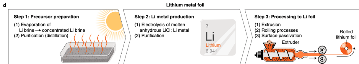
Figure 6.2 Preparation of Li metal foil. 14
