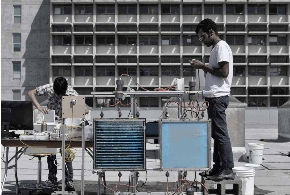
Figure 5.4. Solar PC-T experiments under real solar conditions at subpilot scale. Here, two photoreactors, VIMS (left) and the Planar TiO 2 (right) are in operation during a rooftop experiment in Berkeley, CA.
