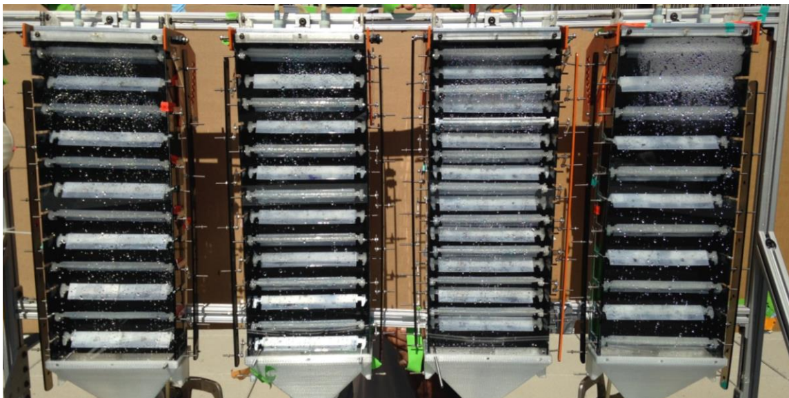
Figure 4.3. VIMS Photoreactor experimental setup in real sunlight conditions. Four separate photoreactors, each with independent reservoirs, distributors, and flow lines, are aligned in parallel on a west-facing rooftop.
