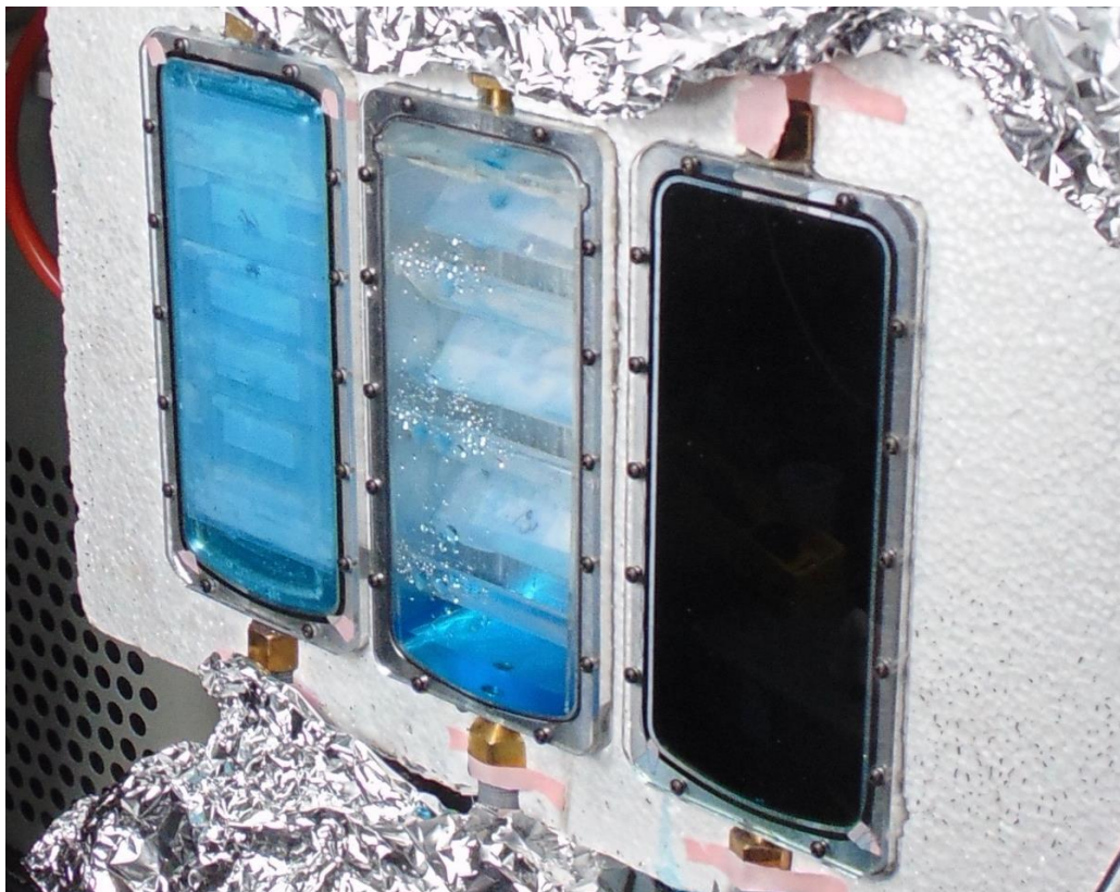
Figure 5.6. Solar PC-T experiments under simulated solar conditions at laboratory scale. Here, three photoreactors, Planar TiO 2 (left), VIMS (center), and Absorber-backed (right) are in operation under simulated solar irradiance in a laboratory setting. All three reactors are housed in a tight-fit insulation manifold.
