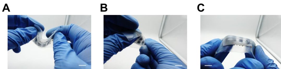
Figure 3.12. Photos demonstrating the conformity of the hydrogel on the BSC.
