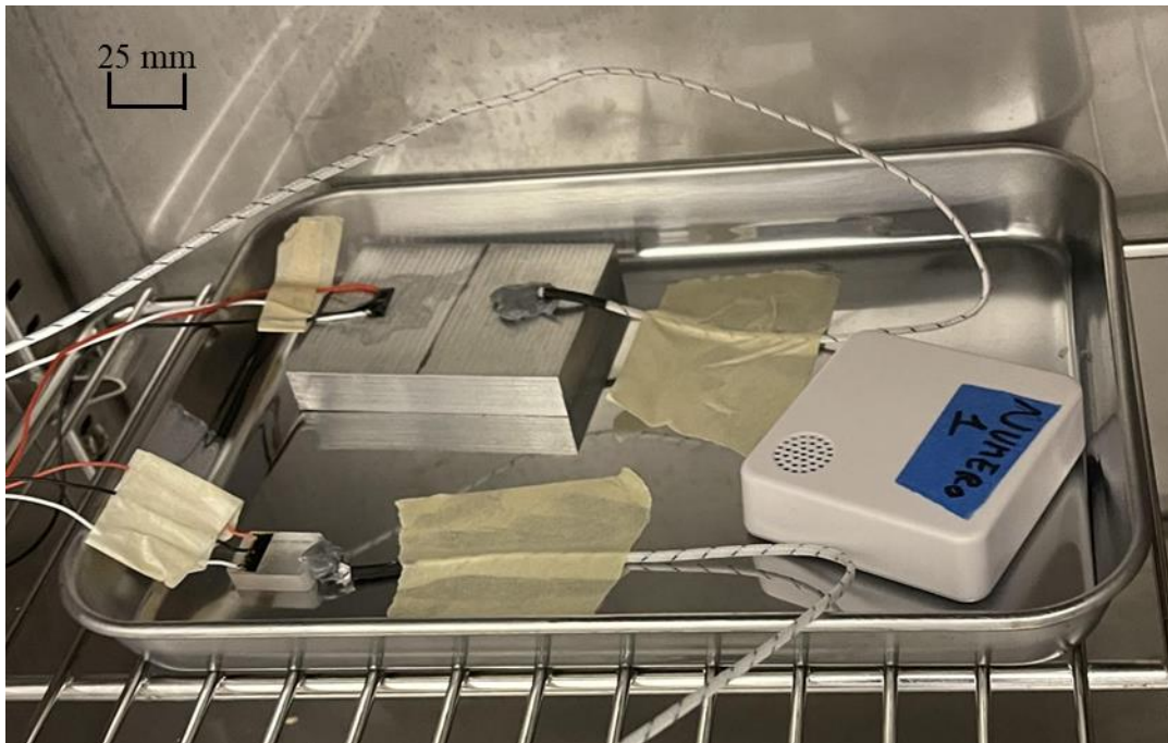
Figure 39. Aluminum 6061 CTE validation test run experimental setup.
