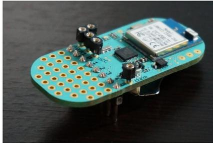
FIGURE 4.4: LightBlue Bean Microcontroller
