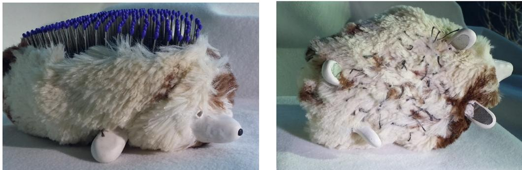
(A) Front of hedgehog, the button-nose, LED eyes, flexible hairbrush back are visible (B) Underside of the hedgehog, conductive clay paws and conductive pet sensor belly are visible
