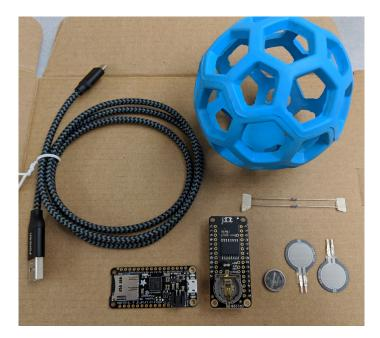
FIGURE 5.3: Core hardware components used in the first iteration of the ball. From left to right: MicroUSB cable, Adafruit Feather M0 microcontroller and RTC add-on w/ battery, JW Hol-ee Roller dog toy, 1K Ohm resistors, and Round Force-Sensitive Resistors. Not pictured, fabric cover and silicon-coated wires.
