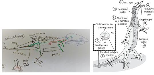
(A) Initial sketch of the dragon design(B) Final detailed diagramFIGURE 4.10: Dragon design sketches
