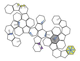
FIGURE 5.4: Flattened diagram of the final sensor placement around the surface of a mixed hex/pentagram ball. For a full life-sized version see supplemental materials, feel free to print, cut and assemble your own ball!
