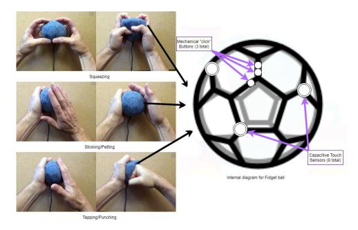
FIGURE 5.1: Sensors embedded in the surface of the Fidget Ball can sense a variety of sensory inputs.
