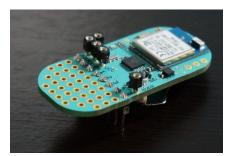
FIGURE 4.4: LightBlue Bean Microcontroller
