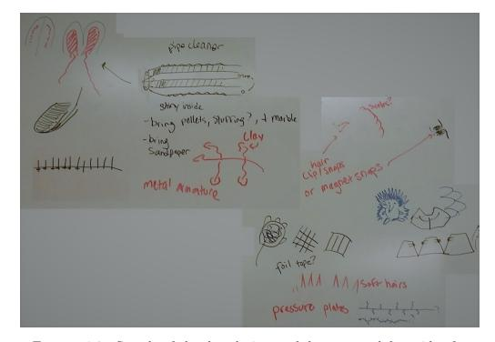
FIGURE 4.3: Sample of sketches during workshop, upper left an idea for using pipe cleaners and stuffing to create a pressure sensor in the style of rabbit ears. Lower left walks through using copper tape and magnets as connectors, and using ideas from soft-robotic designs to create a folding sensor.
