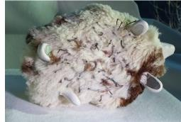
(A) Front of hedgehog, the button-nose, LED (B) Underside of the hedgehog, conduceyes, flexible hairbrush back are visible
