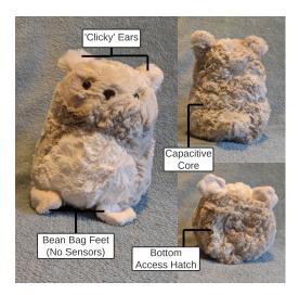
FIGURE 4.20: Diagram showing key features of the final commercial design.
