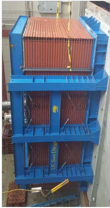
c) Laminar Box on Shake Table
