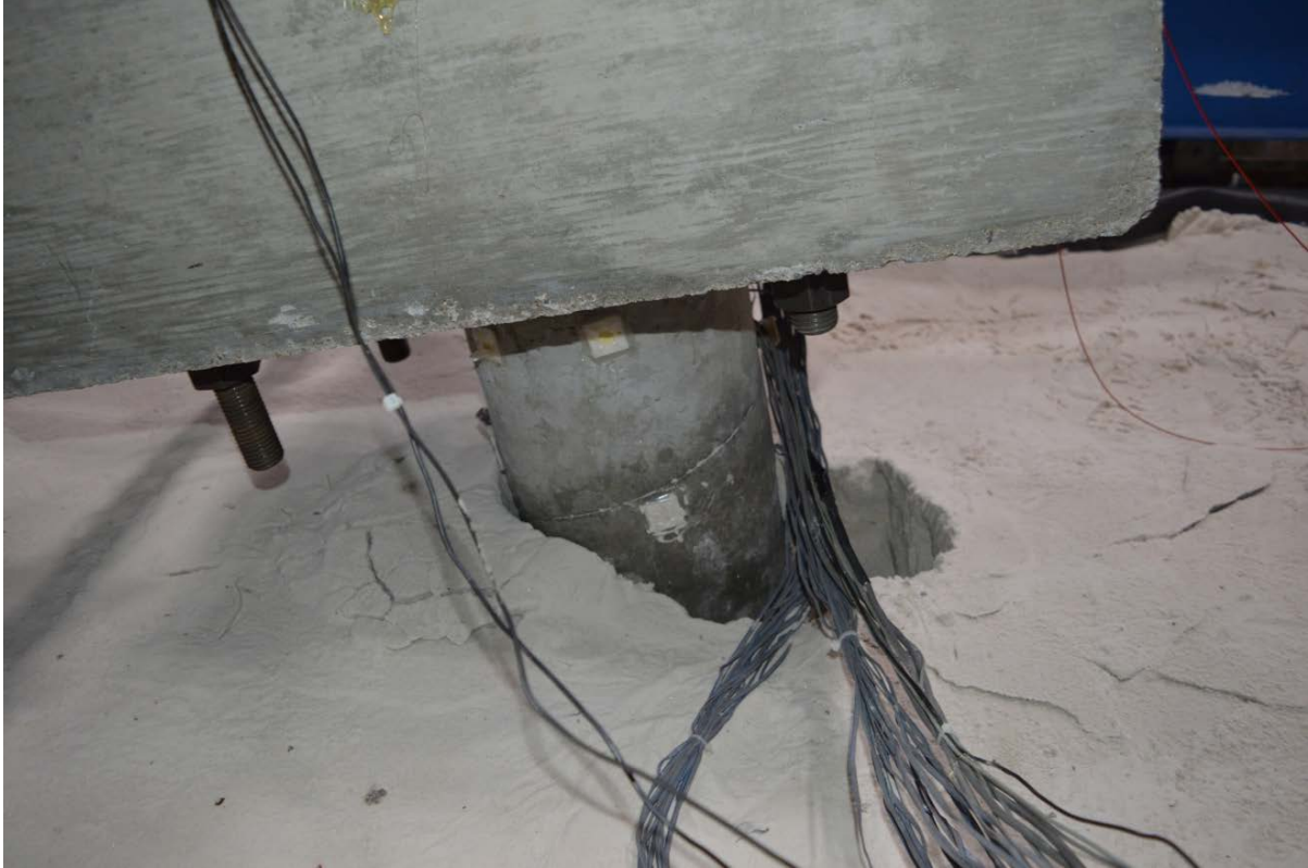
Figure 9-24. Final permanent deformation of the pile head supported by downslope soil
