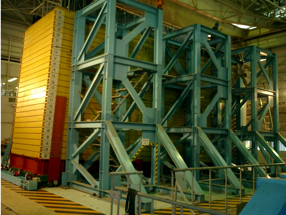
Figure 6-1. Mildly inclined large laminar box on shake table
