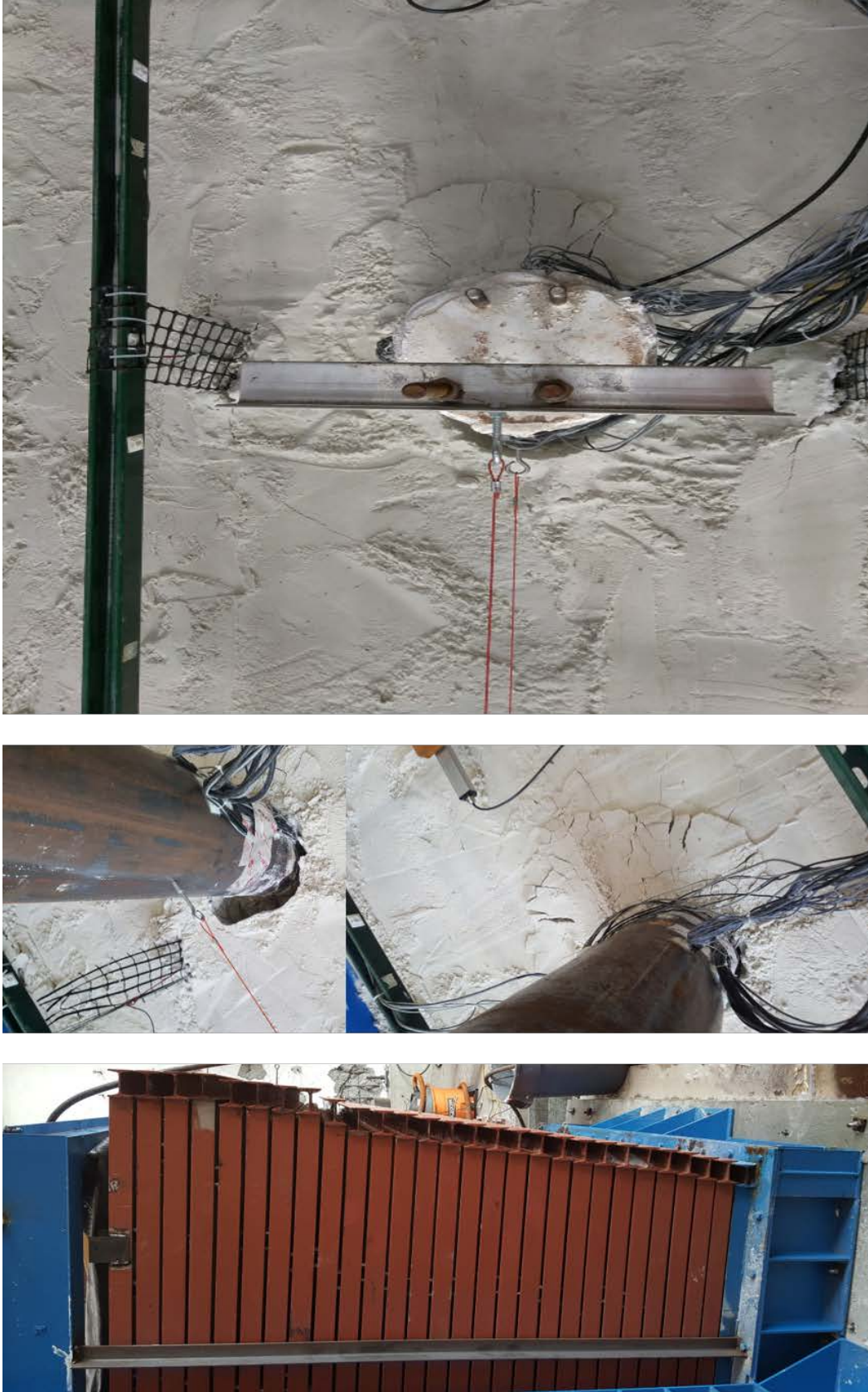
Figure 8-11. Deformed box shape and soil surface after shaking (Upslope cracking and downslope gap formation in the crust)
