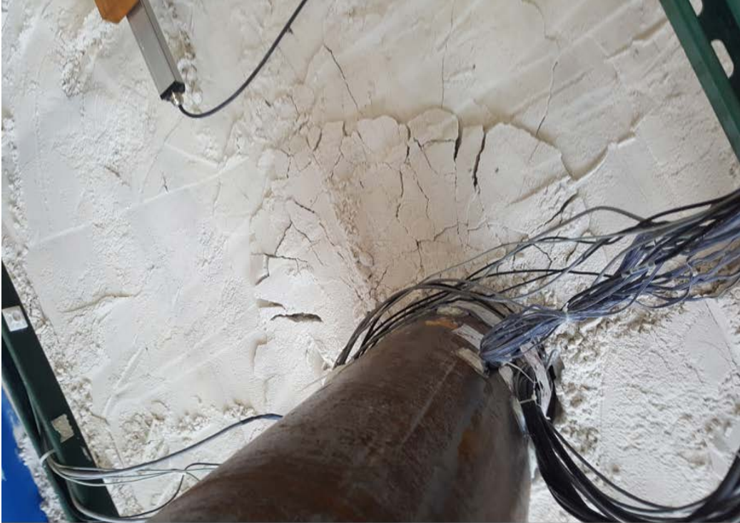
Figure 7-14. Upslope cracking and downslope gap formation in the crust post-shaking (Pictures from Test 3)
