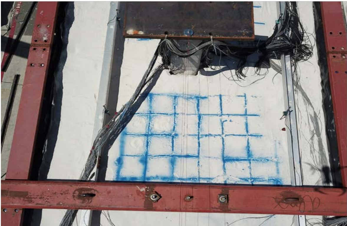
Figure 11-31. Zoomed in soil surface view after shaking (showing upslope heave and downslope gap)
