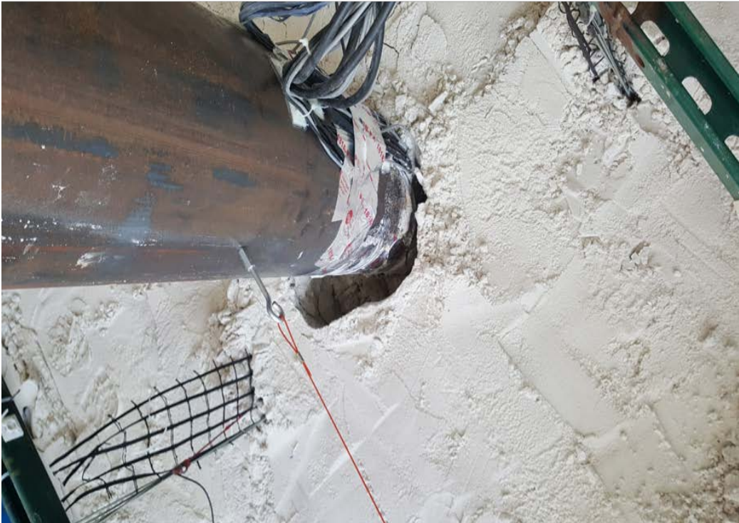
Figure 7-14. Upslope cracking and downslope gap formation in the crust post-shaking (Pictures from Test 3)
