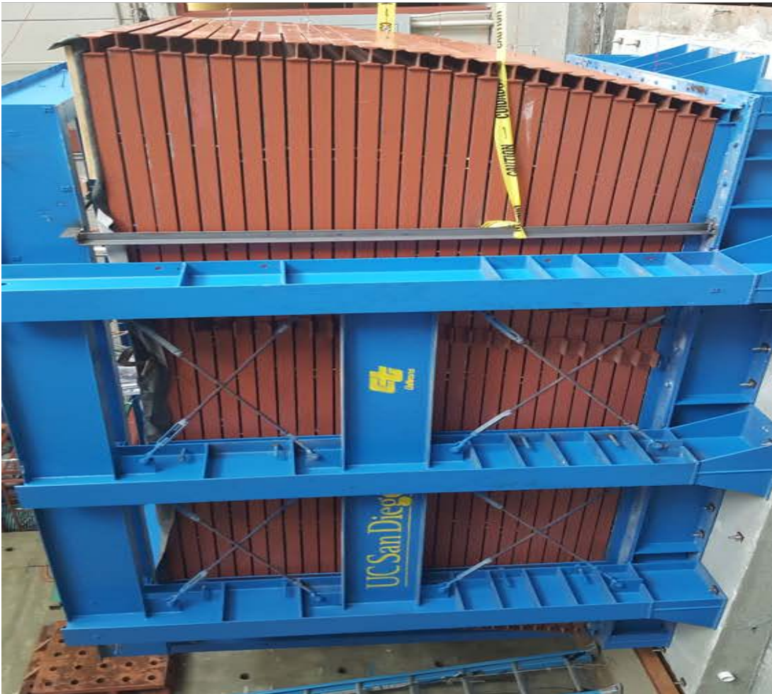
Figure 7-6. Soil box deformed shape and soil surface after shaking in Test 1
