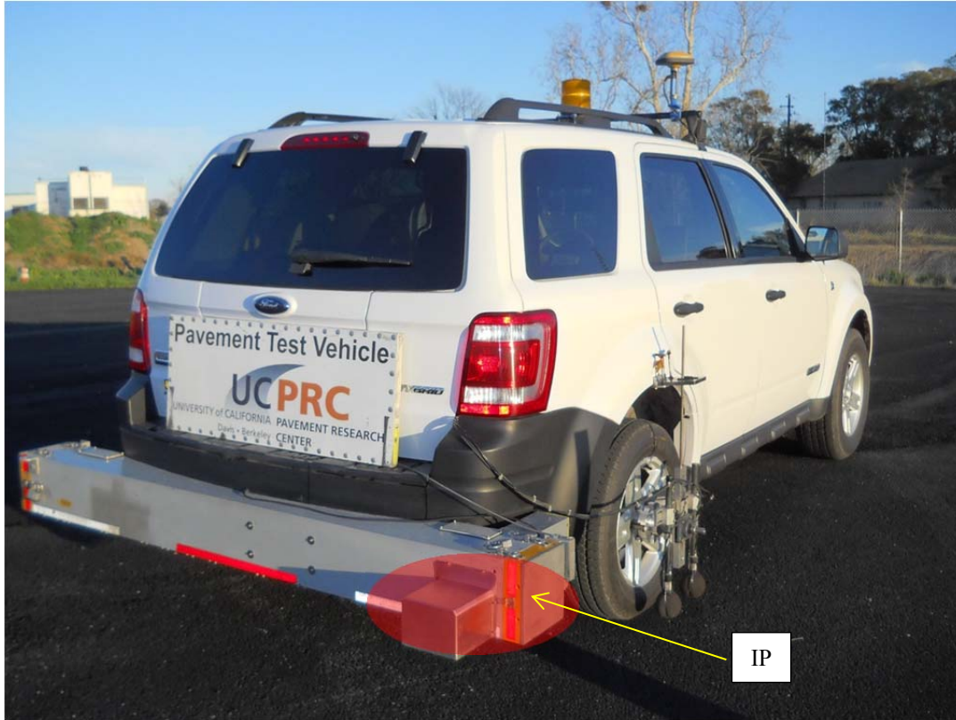
Figure 4.7: Instrumented vehicle with an inertial profiler (IP).
