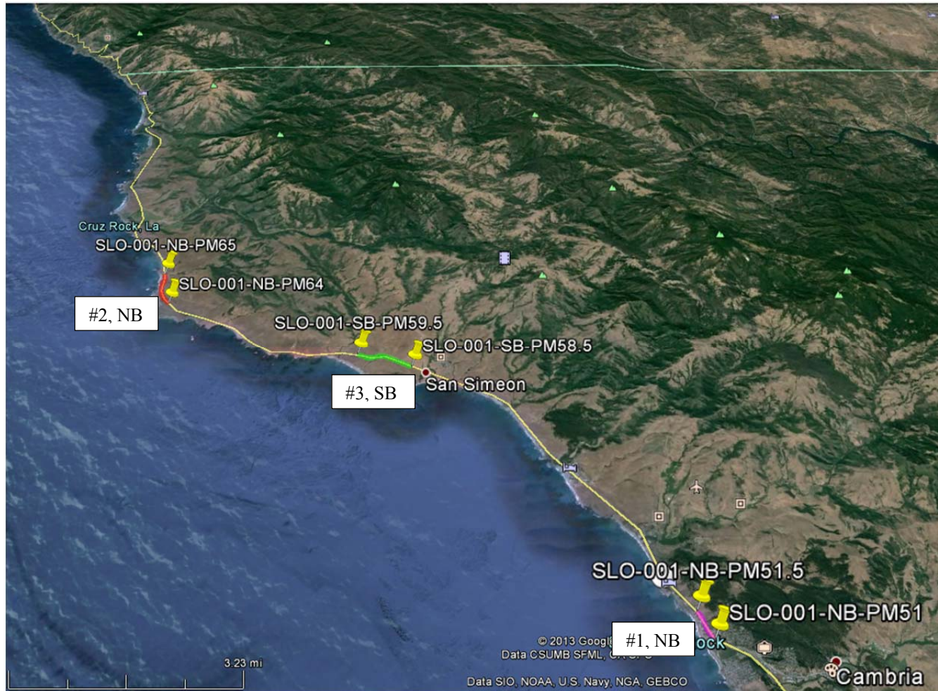
Figure 3.3: Subsections on SLO-1 used for the three bicycle ride quality surveys. (See Table 3.4 for section details.)
