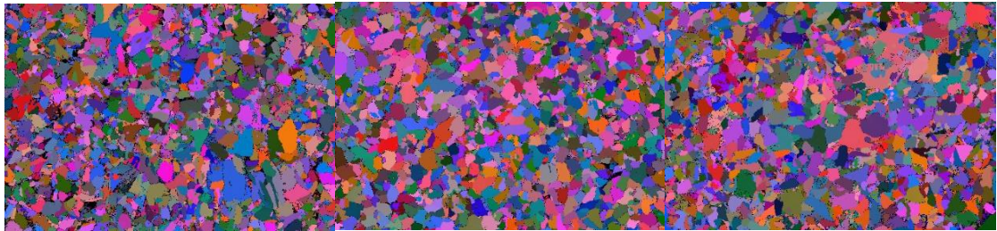
Fig 3.24: Euler color maps of steels heat treated at 1050°C
