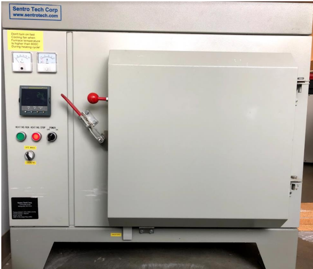
Fig 2.1: ST-1500C-121216 High Temperature Box Furnace
