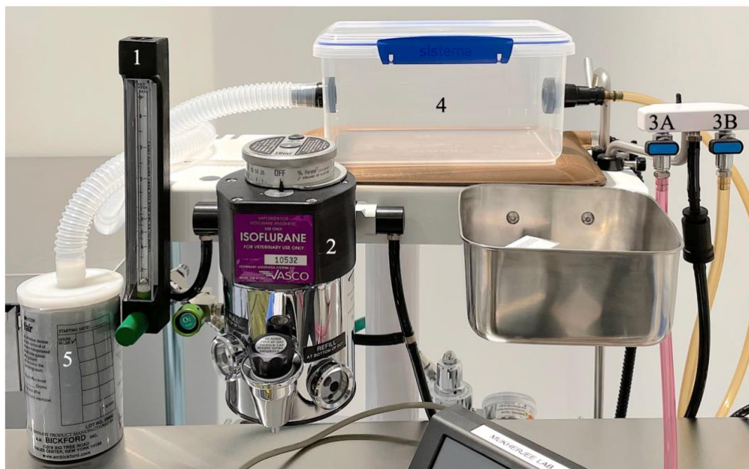
Figure IV.B.1.2. Area 1: anesthetic supply. (1) Airflow meter (2) Isoflurane vaporizer (3A) Pink tubing flowing isoflurane from dual manifold to the stereotax (3B) Yellow tubing flowing isoflurane from dual manifold to (4) induction chamber (5) activated charcoal trap for isoflurane waste.
