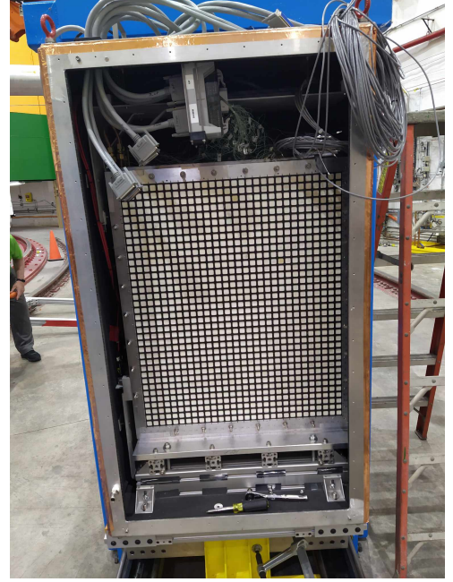
Figure 1: Front view of the Neutral Particle Spectrometer (NPS). The NPS comprises a 36 \times 30 matrix of \text{PbWO}_4 crystals and is placed inside a black box to prevent light leakage.
