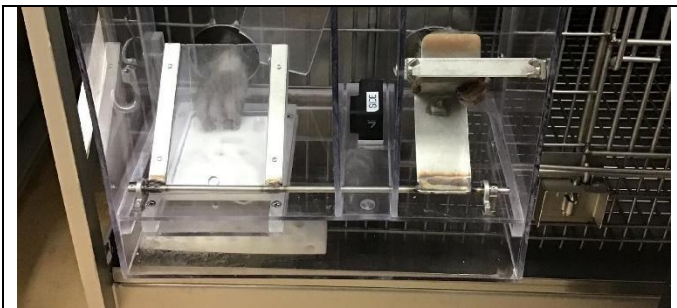
Figure 1.2. Brinkman box. Animal performing the Brinkman board task using the behavioral setup. The lever must be pushed by the left hand in order for the right hand to access the Brinkman board.
