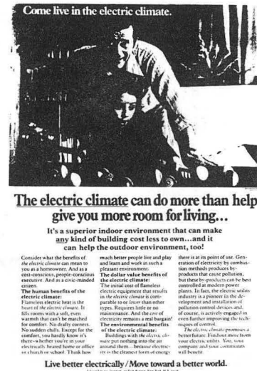
Fig. 114. Huh? This kind of electrical heat requires twice the total energy of natural gas or an electric heat pump. From a national magazine in 1972. (XFB 744-4358)
