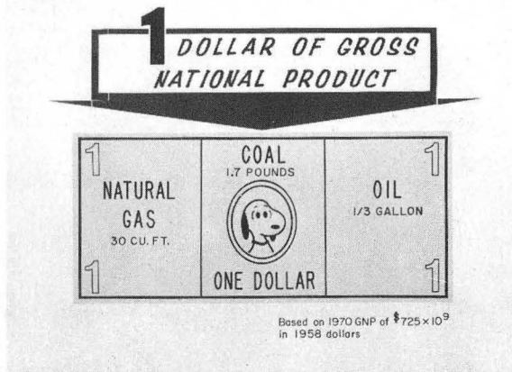
Fig. 57. It took this much energy to produce a buck's worth of GNP in 1970. But we can do better. Dollars are just paper; energy is real! (Author's apologies to Schultz, GNP in 1958 dollars, data from Ref. 34.)
