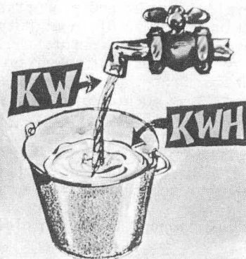
Fig. 19. Power is "how fast", while energy is "how much." (From Honeywell Corporation.)
