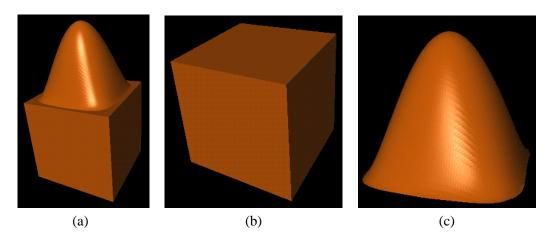
FIGURE 2: A trivariate solid: The complete solid is shown in (a); The boundary face patches are shown in (b); and the implicit boundary surface is shown in (c).
