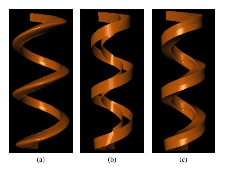
FIGURE 3: Image (a) shows the implicit boundary surface swept along the helical path. Image (b) is the locus of characteristic curves of the boundary face patches along the path. Image (c) shows the swept edges of the image boundary patches. The resulting envelope is the union of these surfaces.
