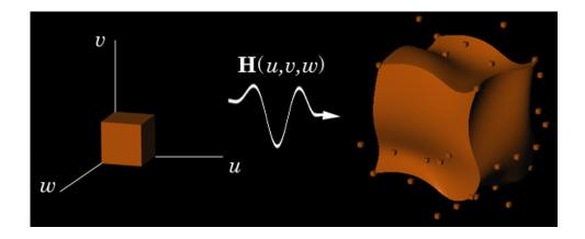
FIGURE 1: A trivariate tensor-product Bézier Solid H(u, v, w) shown with 64 control points (most of which are inside the solid).
