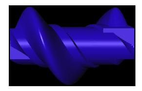
FIGURE 7: Image is the swept surface of the trivariate solid rotating a total of 360° along a horizontal path.
