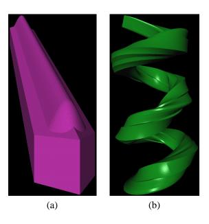
FIGURE 4: Image (a) is the swept surface of the trivariate solid from Figure 2.1 along a diagonal. This is an example of an upright sweep. In image (b), the same trivariate solid is swept along the helix from Figure 3, except in a rotating sweep. The total amount of rotation is 360°.
