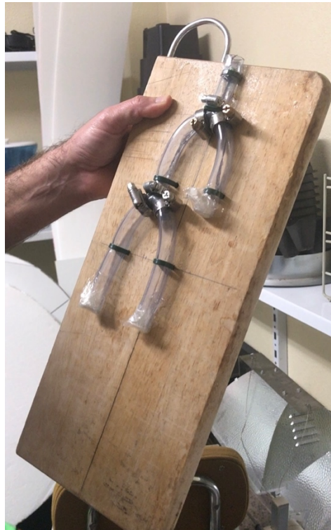
Photo 8. One of Paco’s early experimental prototypes, a double Y-maze affixed to the back of a cutting board he “borrowed” from his house. The mummified remains of a Maize root can be seen in the upper Y of the maze.
