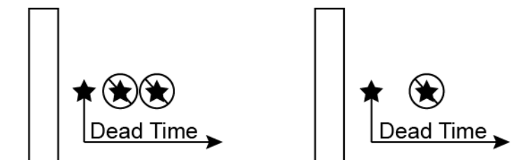
Figure 3.15: Pile-up effect in single photon counting detectors. The square wave indicates the excitation pulse train and the stars are photons incident on the detector. The first photon is detected while photons reaching the detector during the resulting dead time are not.
