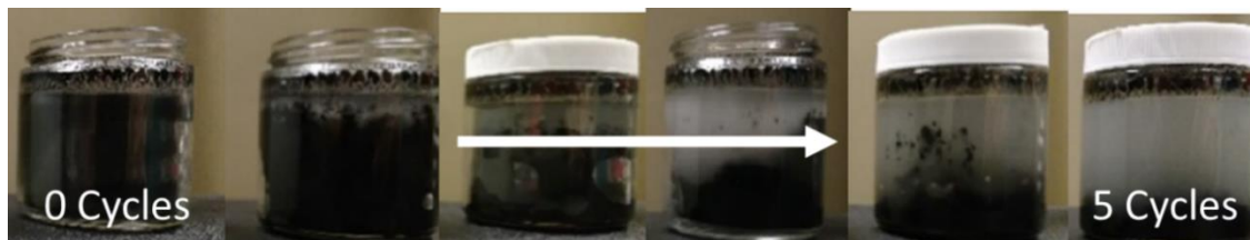
Figure 1.9 Multiwalled carbon nanotubes (MWCNTs) dispersed in paraffin wax. After 5 melt and resolidification cycles, the MWCNTs show a distinct separation and settle at the bottom of the container while the paraffin remains on top. 57 (Adapted and reproduced with the permission of Springer Nature).
