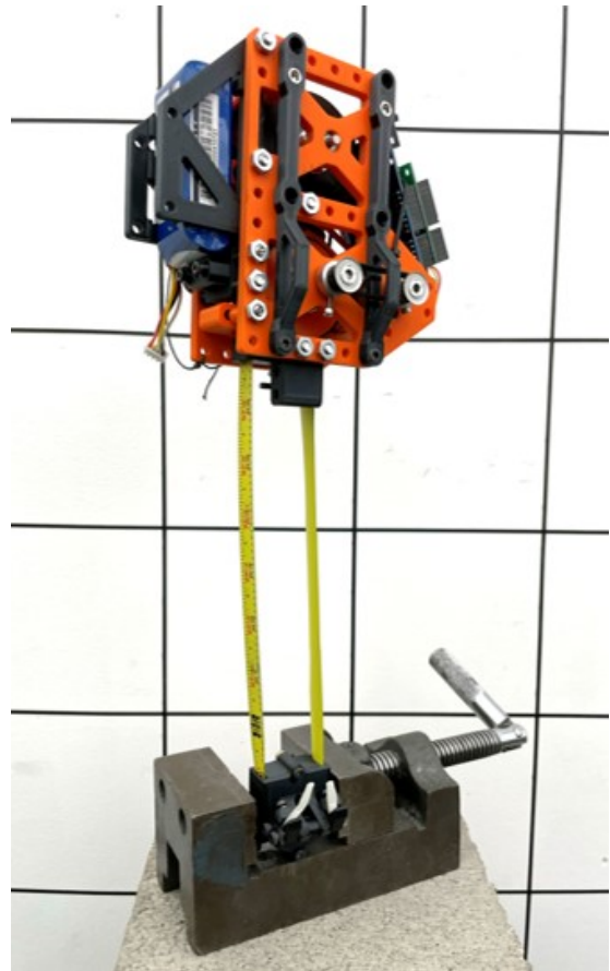
FIGURE 9: EEMMMa-1 STANDING DEMONSTRATION. THE LIMB IS DEPLOYED DOWNWARD, WITH THE END EFFECTOR SECURED IN A VICE. THE WEIGHT OF THE MAIN BODY LOADS THE LIMB IN COMPRESSION, SIMILAR TO A WEIGHT-BEARING LEG.
