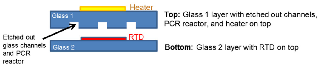
Figure 31. Cross-sectional view of the bioprocessor chip.
