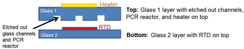
Figure 84. Another cross-section of the microfluidic chip.
