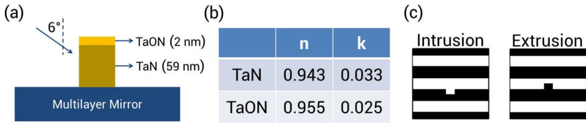
Figure 3.19: (a) Side view of a schematic diagram of EUV mask pattern: absorber pattern height and illumination orientation. (b) Optical properties of the absorber materials at EUV wavelength (13.5 nm). (c) Top-down view of intrusion / extrusion defect definition: Black is the absorber and white is the spacing.
