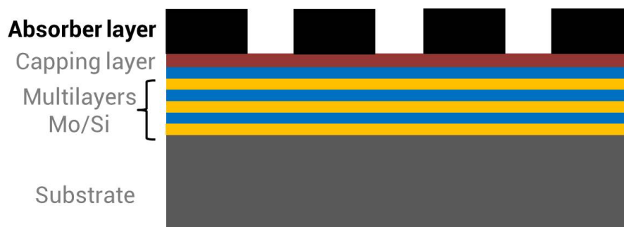
Figure 3.2: Schematic diagram of EUV mask.
