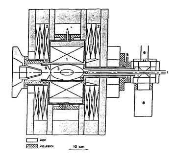
Fig. 1. Elevation view of the CAPRICE- $2\omega_{CE}$  source. (1) shows the sextupole magnet. (2) shows the solenoid magnets. (3) shows a inner elipse where the ECR resonance condition is met. On the outer elipse the magnetic field is twice as great. (6) shows RF waveguide which feeds into a transition section. (10) shows the end of the coaxial coupling.
