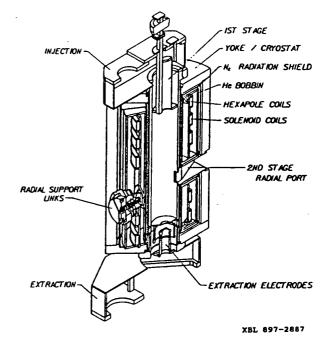
Fig. 2. Elevation view of the LBL AECR. This Nd-Fe-B sextupole has radial slots for pumping the plasma chamber. RF power is fed by a transition from rectangular to round waveguide.
