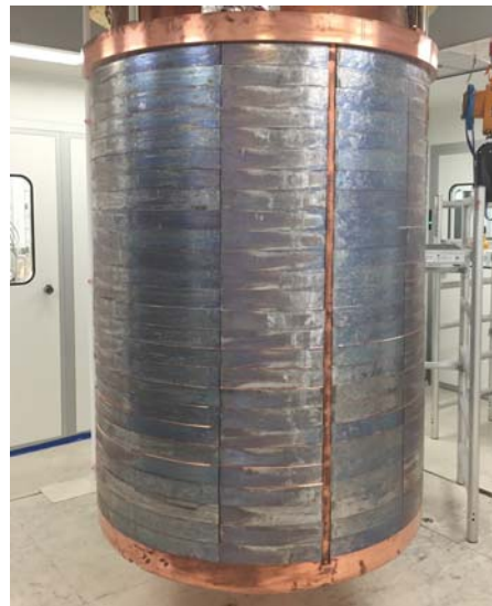
Figure 4. Roman Lead lateral shield, which surrounds the towers.
