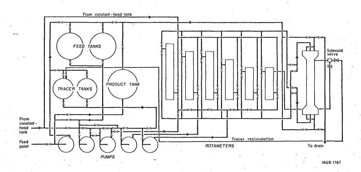
Fig. 7. Layout of flow system.
