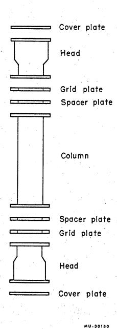
Fig. 1. Exploded diagram of column assembly.
