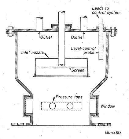
Fig. 5. Diagram of column head.
