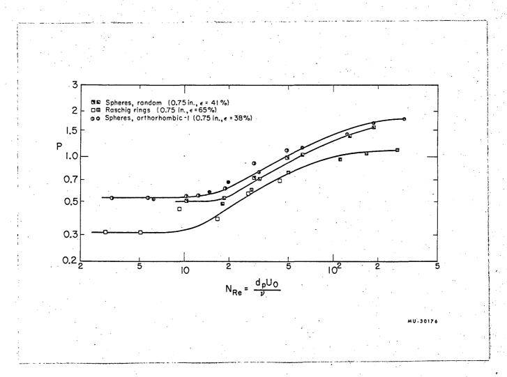
Fig. 8. Influence of viscosity. (In the legend, the symbols on the left are for glygrol-water mixture and those on the right for water alone)
