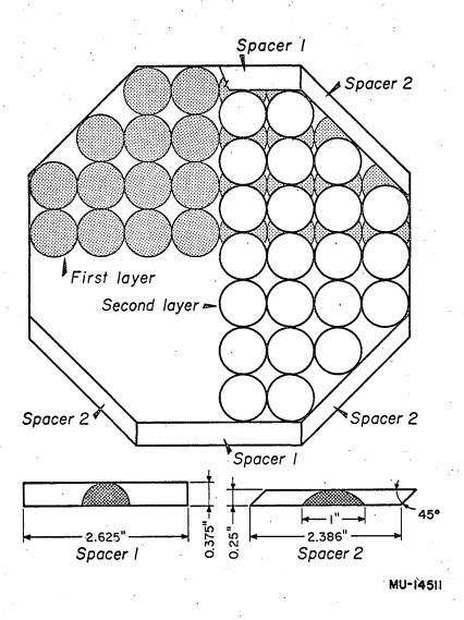
Fig. 3. Arrangement of packing and spacers, column 2 (orthorhombic-1, octagonal).
