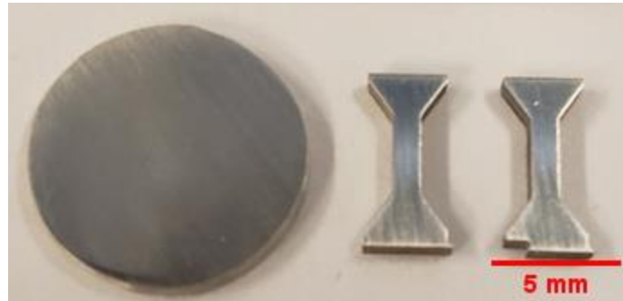
Figure 1: 10mm diameter silver alloy disc post-HPT with two small-scale dogbone samples.
