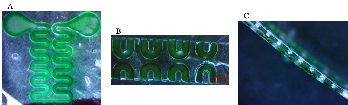
Fig. 3.16 Manufactured Channel Sensor. A. The channel sensor formed in epoxy is filled with dye (green) and enzyme hydrogel (clear) and coated with a 10 micron layer of NuSil. B. Then the sensor is chopped to individuate the channels and expose entrance holes on the side. C. Side view of sensor, showing entrance holes.
