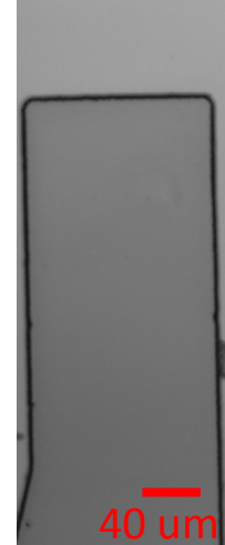
Fig. 3.12: Single Reaction Chamber. One reaction chamber formed by photolithography in SU-8 on a silica wafer
