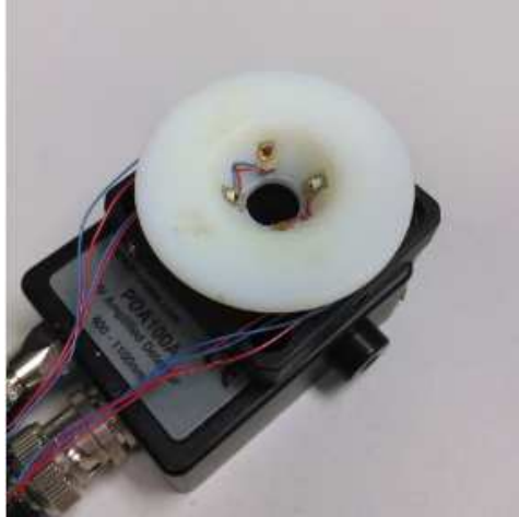
Figure 2. The probe: Lactate and oxygen sensitive lifetime measurements are made by exciting an implanted sensor with LED light and by collecting the sensor's excited light emission on a photodetector. A long-pass optical filter between the LEDs and detector is used to prevent LED light from saturating the detector. LEDs are attached to a custom 3D printed conical mount in order to aim their output light onto a sensor implanted in subcutaneous tissue.
