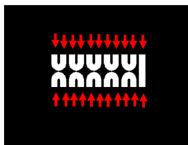
Fig. 3.15 Channel Sensor Chopping. The 'channel sensor' is chopped with a razor along the lines drawn in red, individuating small chambers and exposing an entrance for analyte to diffuse into on the side (direction of analyte diffusion indicated by red arrows).
