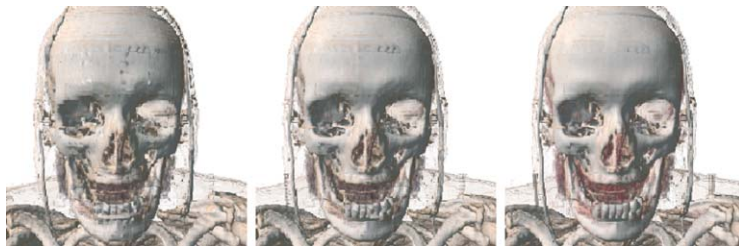
Fig. 7. Comparing image quality for interactive rendering of the visible human male data. Left: low quality, 7.1 fps. Middle: medium quality, 5.4 fps. Right: high quality, 2.8 fps. Images are provided by Stefan Guthe at WSI/GRIS, University of Tübingen.
