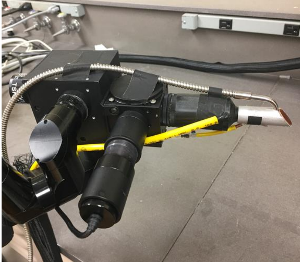
Figure 2: Image of the clinical handpiece and probe head
