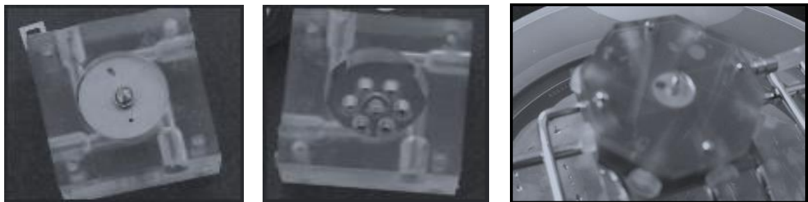
Figure 2-4: Test turbines. (Left and middle) Top and bottom view of the 1 cm rotor in a 1.6 cm cubic turbine with four tangential nozzles at 90 degree spacing. (Right) A 4 cm octagonal turbine with eight nozzles, used for testing the four rotors at eight nozzle configurations.
