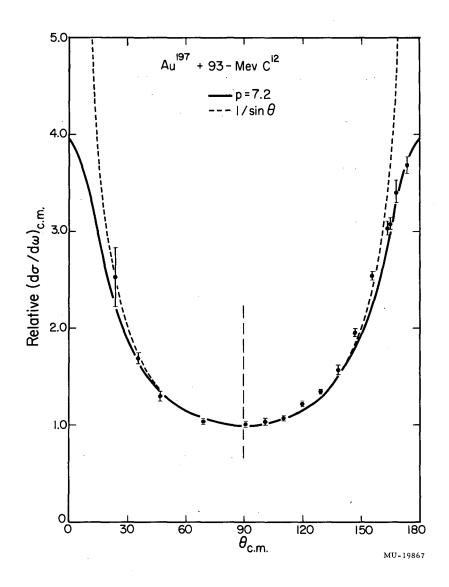
Fig. 6. Center-of-mass angular distribution of fragments from fission of Au<sup>197</sup> induced by 93.3-Mev C<sup>12</sup> ions. The solid curve represents Halpern and Strutinski's theoretical angular distribution with p=7.2 (see text).
