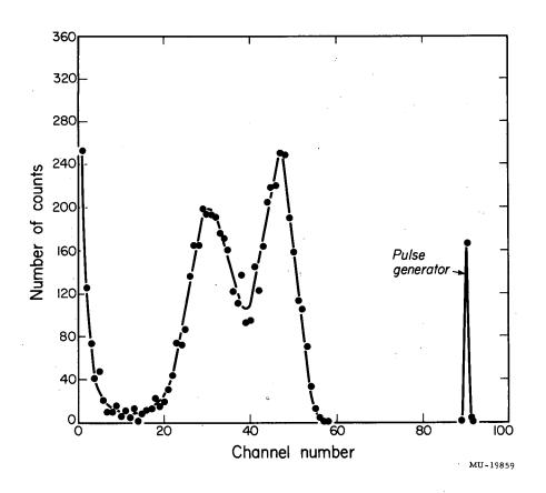
Fig. 3. Spectrum of fragment kinetic energies from spontaneous fission of Cf<sup>252</sup>. Observed with a solid-state detector reverse-biased by 9 v.
