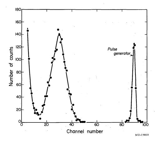
Fig. 4. Spectrum of fragment kinetic energies from fission of Au<sup>197</sup> induced by 93.3-Mev C<sup>12</sup> ions. Observed at 90 deg to the beam with a solid-state detector reverse-biased by 9 v.
