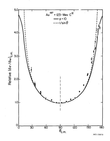
Fig. 5. Center-of-mass angular distribution of fragments from fission of Au<sup>197</sup> induced by 123.3-Mev C<sup>12</sup> ions. The solid curve represents Halpern and Strutinski's theoretical angular distribution with p=10 (see text).
