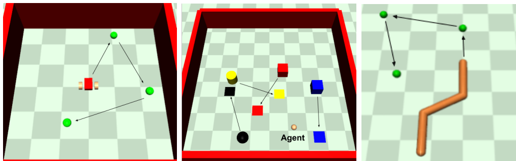
Figure 4.3: From left to right (1) the wheeled locomotion environment with the waypoints depicted in green (2) the object manipulation environment with different objects (blocks and cylinders) and their correspondingly colored goals (squares) (3) the swimmer navigation task with the first 3 waypoints depicted in green.
