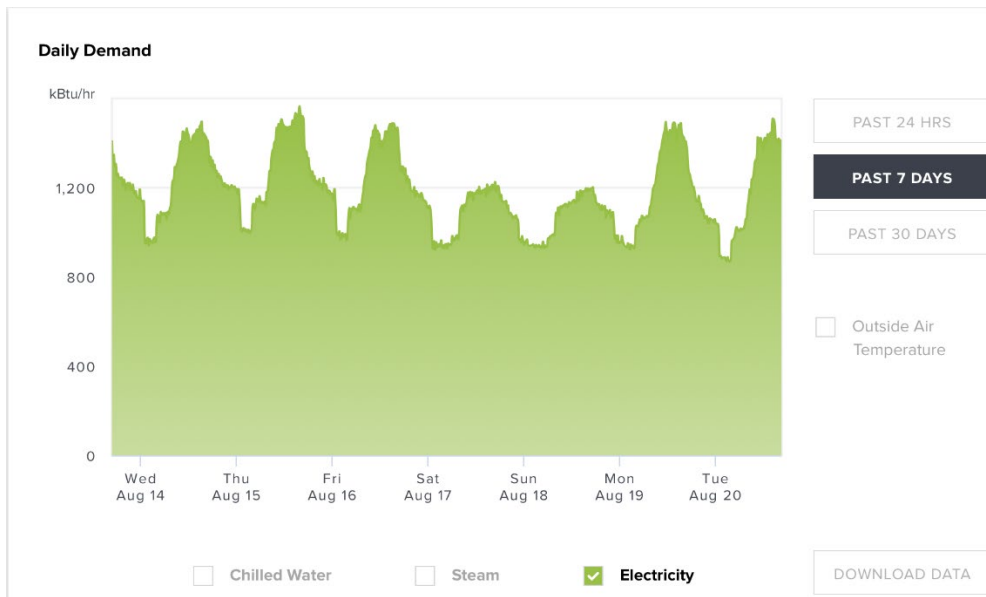
Figure 52: A graph of a week of energy use from Bainer Hall, an engineering building with classrooms, offices, and laboratories [3] Electricity use is available on a daily, weekly, and monthly basis.
