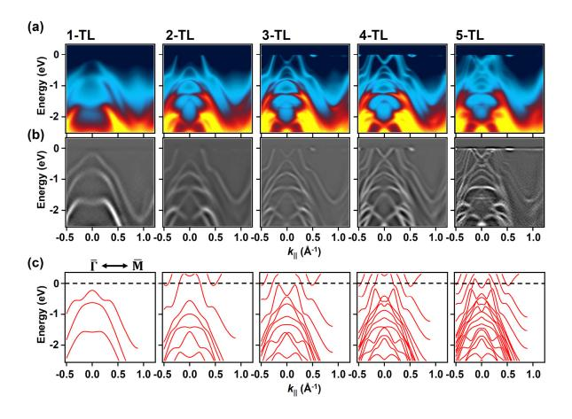
**Figure 4 (a)** ARPES maps along the  $\overline{\Gamma K}$  direction taken from 1-, 2-, 3-, 4-, and 5-TL samples at 20 K using 53 eV photons. **(b)** Corresponding second-derivative maps. **(c)** Corresponding calculated band structures.
