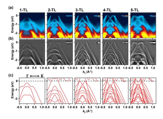
**Figure 5 (a)** ARPES intensity maps at the Fermi level taken from 1-, 2-, 3-, 4-, and 5-TL samples at 20 K using 53 eV photons. **(b)** Corresponding calculated Fermi surface contours. The calculation is for a freestanding slab with no substrates included.
