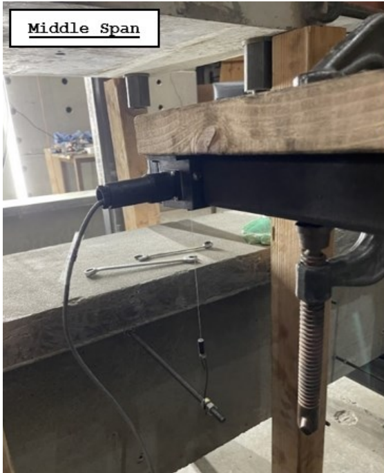
Figure 3-24: Vertical WPs attachment to the beam specimens
