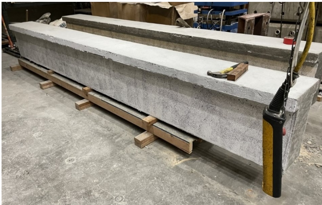
Figure 3-20: Finished large beam specimens with paint for DIC
