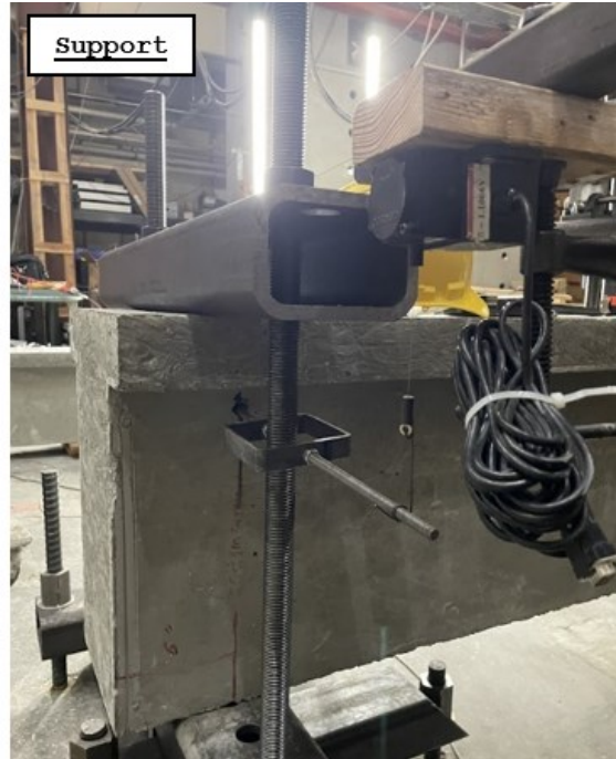
Figure 3-24: Vertical WPs attachment to the beam specimens
