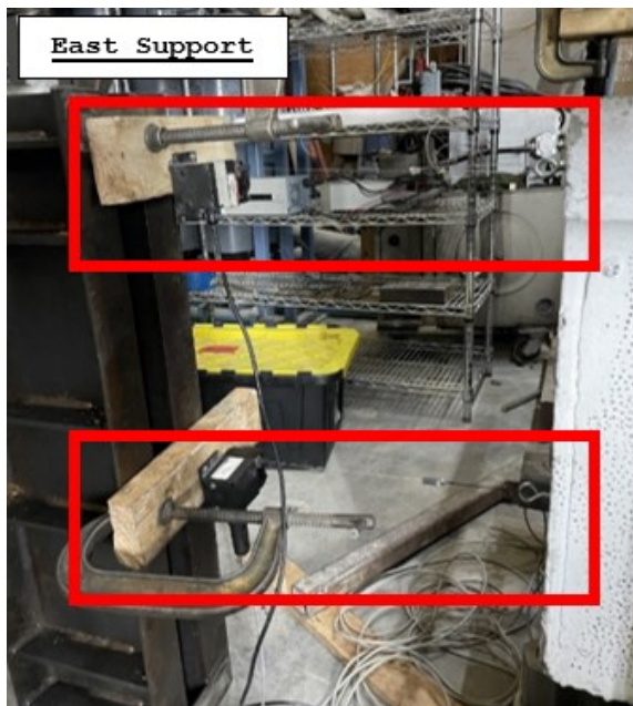
Figure 3-25: Horizontal WPs attachment to the beam specimens
