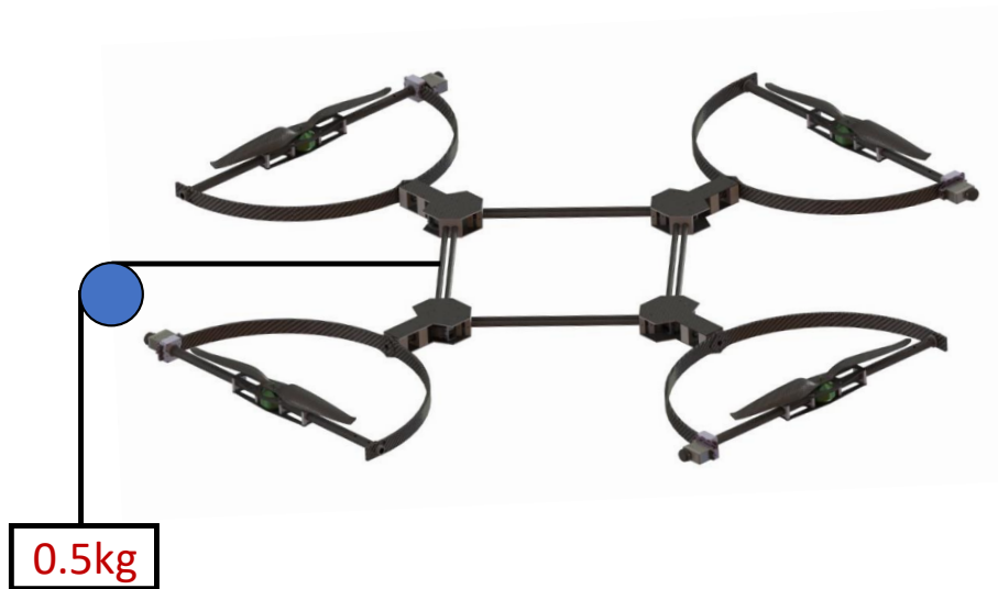
Figure 6.12: Illustration of pulley experiment to apply force in X and Y directions.
