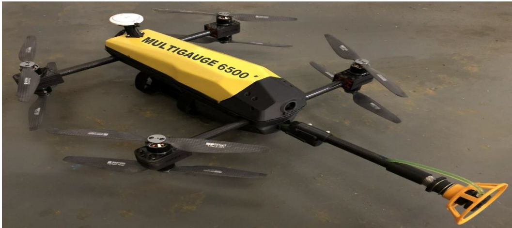
Figure 1.1: Drone with mounted ultrasonic thickness sensor by Tritex NDT.
