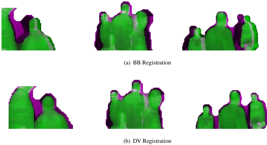
Figure IV.8: Details of registration alignment errors in the bounding box registration approach and corresponding alignment success for the Disparity Voting (DV) Algorithm for several occlusion examples using non-ideal segmentation.
