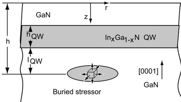
FIG. 4. Characteristic distances for a buried stressor in GaN layer with embedded QW. The sample surface  $z=0$  corresponds to the  $(0001)$  GaN growth plane with the  $z$  axis in the  $[000\bar{1}]$  crystallographic direction.
