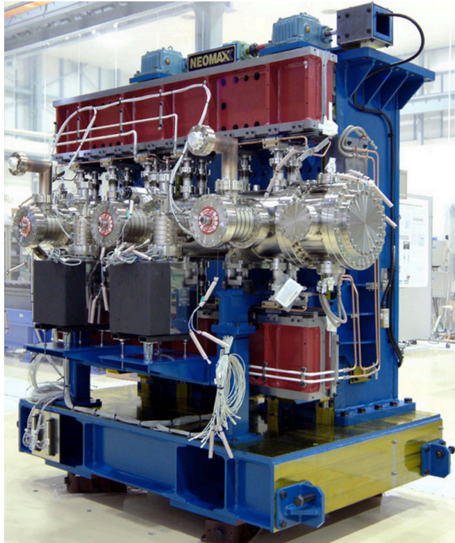
Fig. 2.7 In-vacuum undulator. Image courtesy of ALS, Berkeley Lab.
