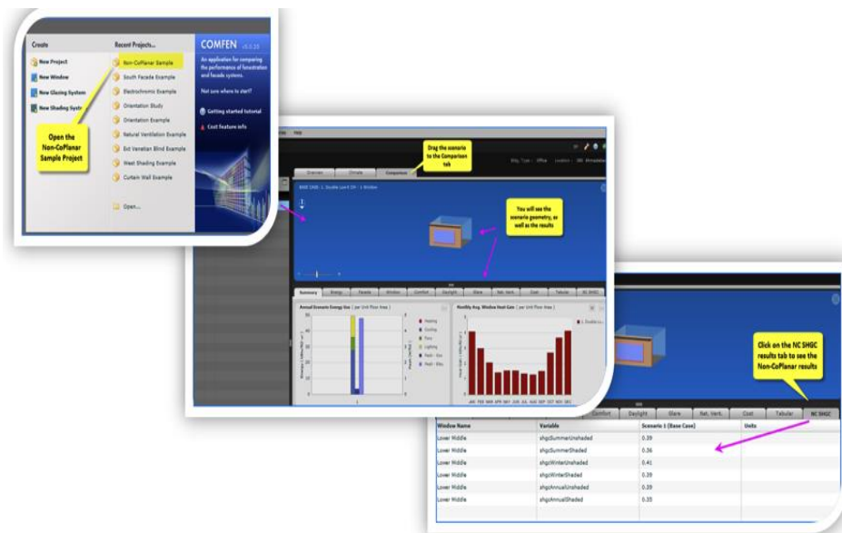
Figure 10: Illustration of a CBERD tool: COMFEN with the non-coplanar shading module integration
