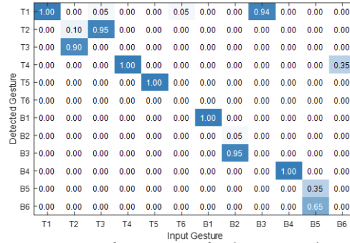
Fig. 17. Confusion matrix for detecting 12 keys.
