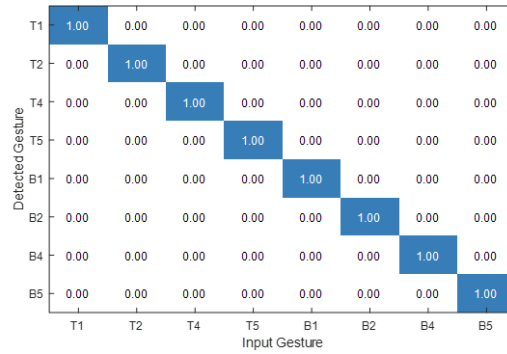
Fig. 19. Confusion matrix for detecting eight selected keys.
