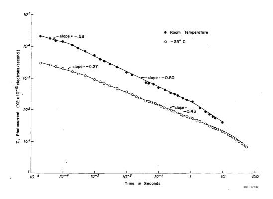
Fig. 4. Log photocurrent versus log time for a metal-free phthalocyanine sample at room temperature and at -35°C.
