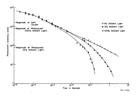
Fig. 9. Log photocurrent versus log time of a metal-free phthalocyanine sample with varying amounts of ambient light.
