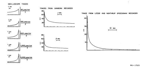
Fig. 3. Typical photoconductivity decay data for metal-free phthalocyanine at room temperature.
