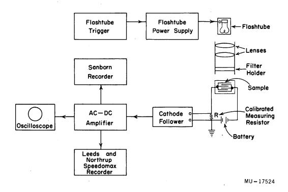
Fig. 2. Block diagram of conductivity apparatus.
