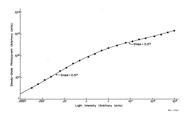
Fig. 6. Intensity dependence of metal-free phthalocyanine steady-state photoconductivity.
