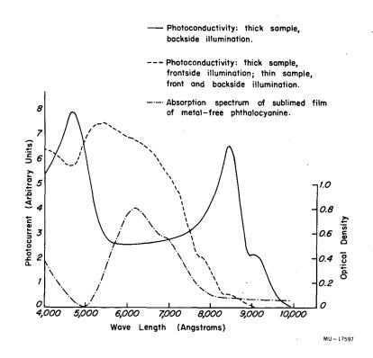
Fig. 8. Spectral response of steady-state photoconductivity and absorption spectrum of metal-free phthalocyanine films. (50 A band width).
