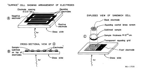
Fig. 1. Diagram of sample cells.
