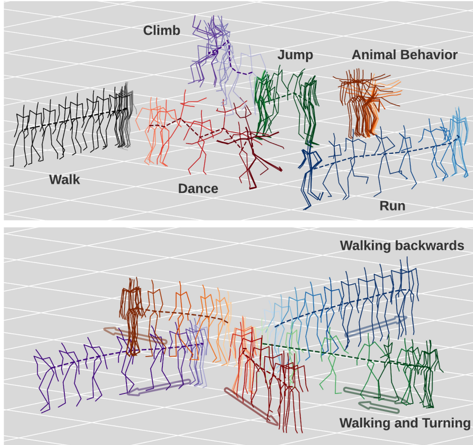
Figure 5.1: ODMO motion generation. Top: Sample motion sequences generated for multiple activities; Bottom: Diverse motion sequences for Walk activity generated by multi-modal sampling.
